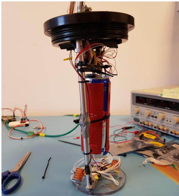
Figure 4-19: The insides of the physical prototype subsea sensor system.
