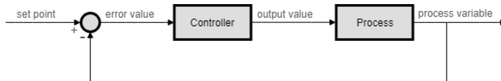
Figure 2-7: Closed loop control system using feedback to steer the output value to the desired process variable, which is the set point value.
