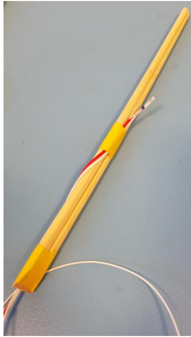
Figure 4-16: Temperature sensor taped to wooden chopsticks.
