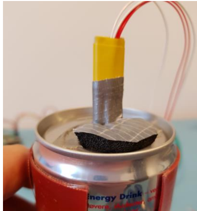
Figure 4-18: Insulation material is fitted into the soda cans opening, to ensure that heated air won't escape easily.
